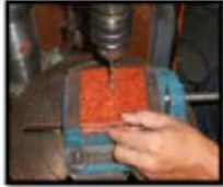
To bore a hole in middle of test specimen
